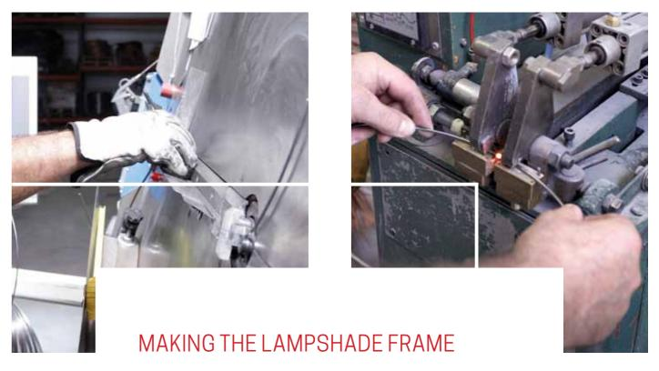
Lampshade frame wires are shaped, spot-joined and welded in our state-of-the-art machine park. Final polishing... and it's time for the first quality inspection. We check the height, shape, angles and welds to eliminate flawed items.
